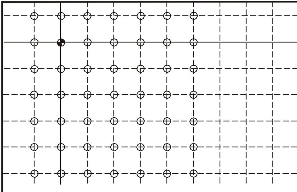
The four corner pedestals are located precisely in position and set level using the 3.6M straight edge and laser or spirit level. The intermediate edge pedestals are then wound up to the straight edge thus establishing their correct level. From the edge pedestals the 3.6M straight edge can now be used to level the pedestals in the centre of the grid. Once all of the pedestals in the block have been leveled the panels are positioned and the process repeated. (FIG 7).
