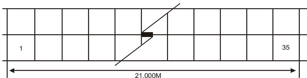
E.G.  $\frac{21.000M}{35 \text{ No panels}} = \text{module size } 600.00mm$
